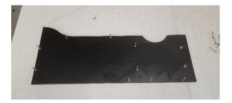
Next, you will put down your large front piece and middle piece with the provided cam locks facing inside. Lock in the cam locks by twisting with a screwdriver.
