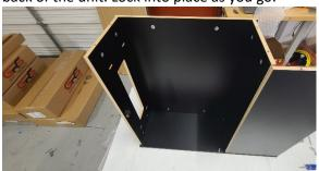
4. The next piece is the back door. This panel will be secured with only one cam screw and the back door clip. This makes it tricky because it can hang, and it will break off. Make sure you are supporting this piece.
